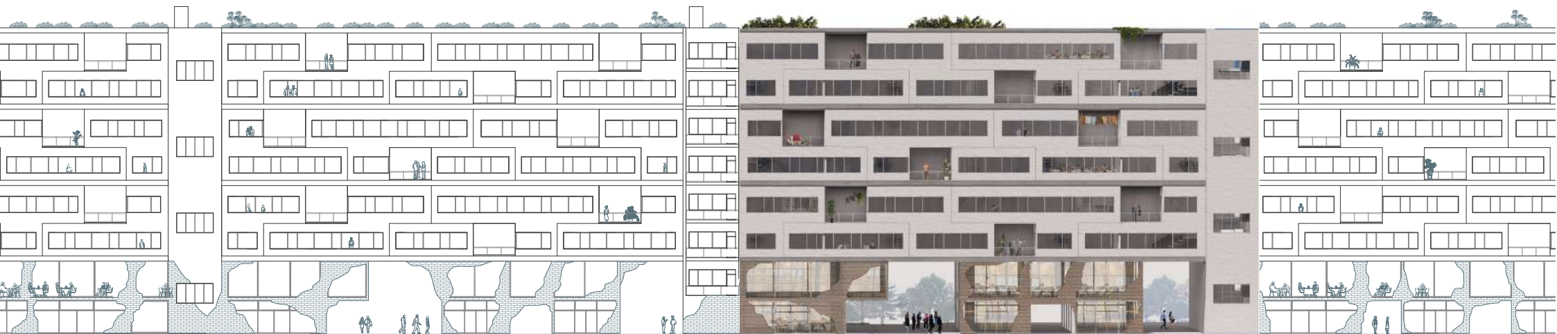
Each building unit has its own vertical circulation area, however the corridors of each unit are connected to its neighbouring building.
